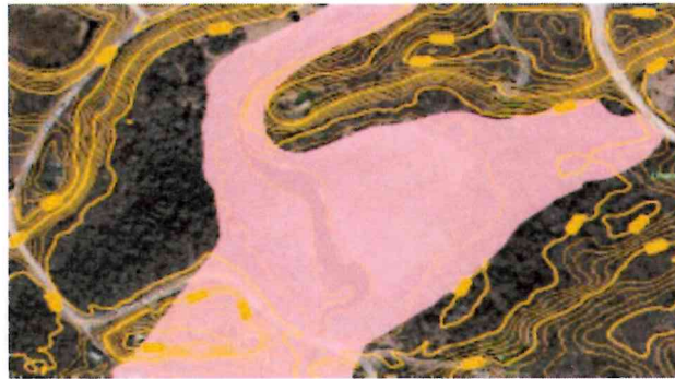
Figure 1. The mapped floodplain may not always align with the on-the-ground contour elevations
